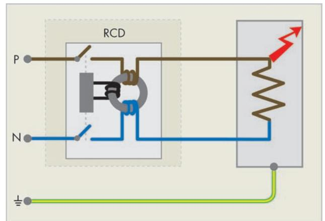
designed, as the current resulting from a fault is generally significantly higher than other protective conductor currents.
