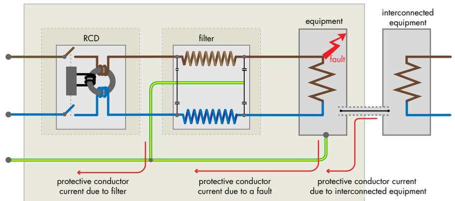
**Figure 2: Protective conductor currents resulting from a filter, a fault or interconnecting cables.**
