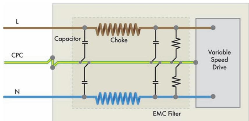
**Figure 1:** A typical filter circuit which includes series connected inductors, bypass capacitors and resistors to discharge the capacitors
