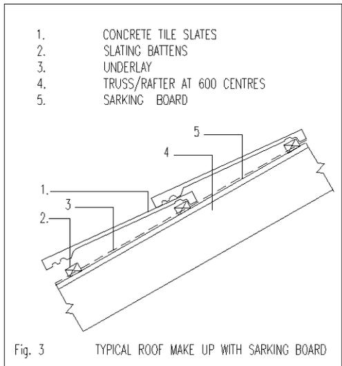
Fig. 3 TYPICAL ROOF MAKE UP WITH SARKING BOARD
