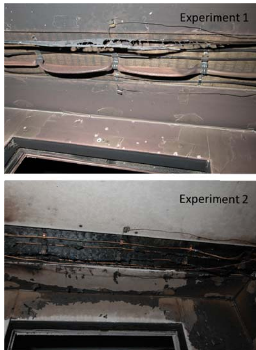
Figure 6 - Comparison of the condition of cables and cable supports after the experiments (In both images the plastic clips have failed but the metal supports are intact)
