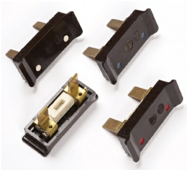
Figure 3.17 A range of BS 3036 rewirable fuses: 5 A (white), 15 A (blue) and 20 A (red)
