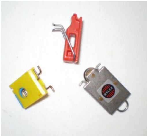
Figure 6.5 Lock-out devices for circuit breakers and RCBOs
