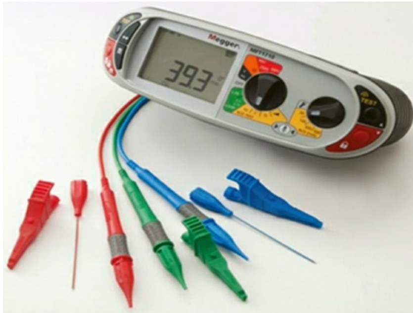
Figure 6.23 Multi-function test instrument showing a range of leads and probes (image courtesy of Megger)
