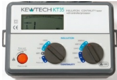
Figure 6.19 Insulation resistance testing – the left dial is set to 500 V and the right dial is set at 2000 MΩ
