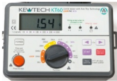
Figure 6.20 Earth fault loop impedance testing – this example shows the dial set at Loop – 20 Ω. Loop 200 Ω and 2000 Ω may need to be used when testing TT systems
