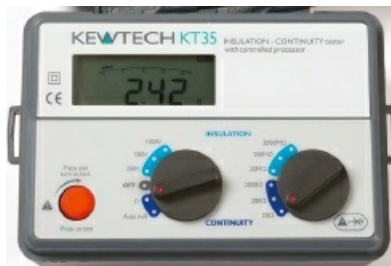
Figure 6.18 Continuity testing – the left dial is set to the \Omega scale and the right dial is set at 20 \Omega
