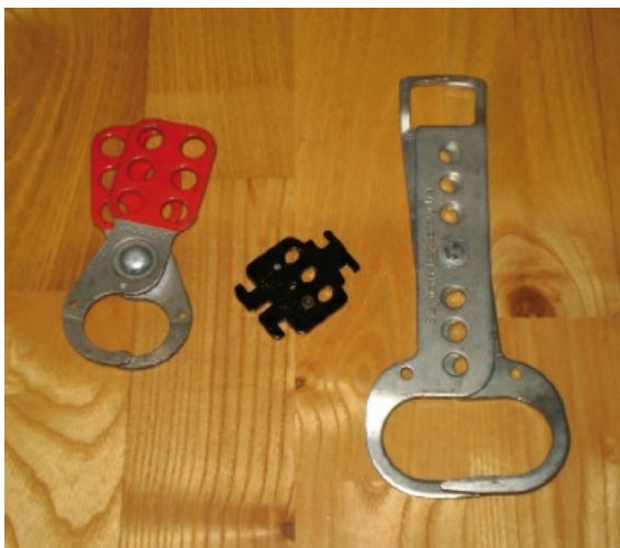
Figure 6.4 Lock-out facility – can be used with one or more locks
