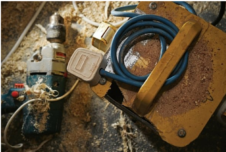
Figure 7.4 Damaged transformer and poorly maintained equipment lead to a high risk of injury
