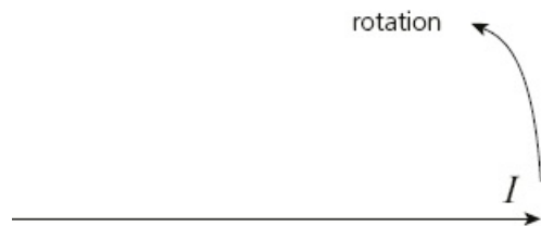
Figure 2.38 Constructing a phasor; using a reference line
