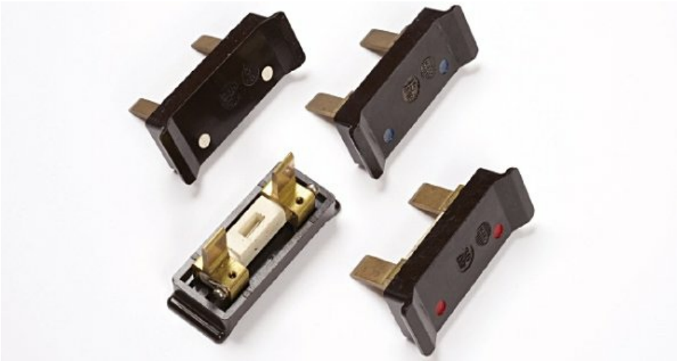
Figure 2.95 A range of BS 3036 rewirable fuses: 5 A (white), 15 A (blue) and 30 A (red)
