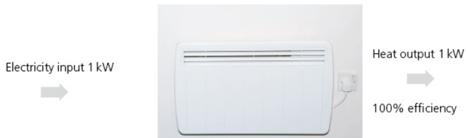
Figure 1.10a The efficiency of an electric panel heater
