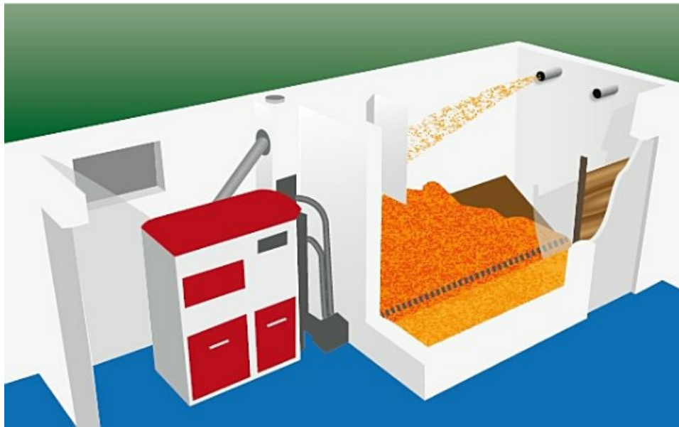
Figure 1.19 Biomass boiler with suction feed system
