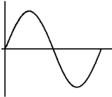
The frequency of the sine wave is the number of cycles that occur every **second**. The periodic time of one cycle can be found by dividing the frequency by one second.
