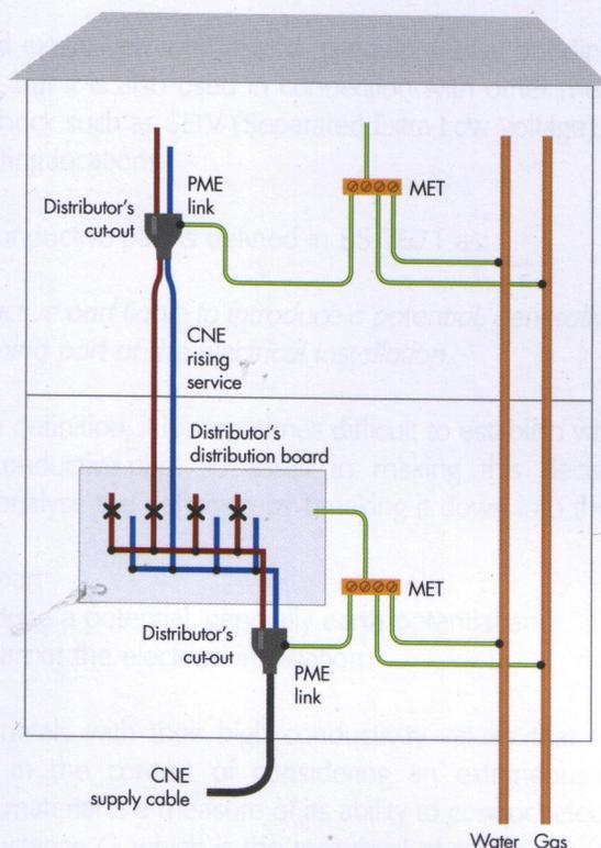
► **Figure 5.17** Typical main bonding arrangement in a small office block
