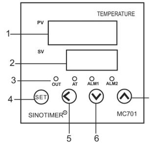
1. PV display window, to display the measured values
