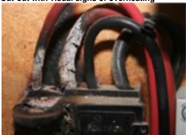
Cut-out with visual signs of overheating
