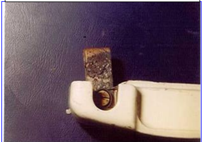
Photo example: Pitted blade, due to making poor contact:
