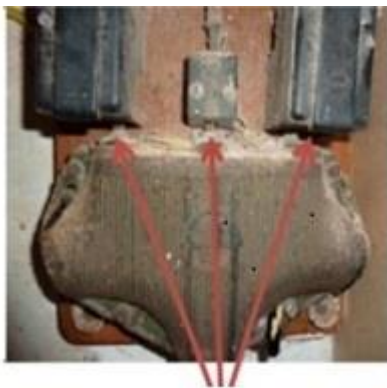
Visible bare conductors
