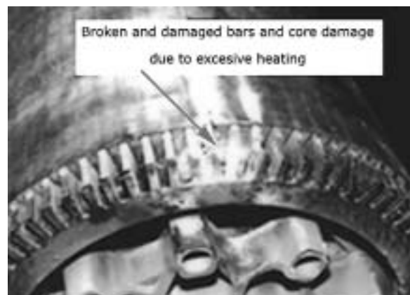
Figure 10. Food Mixer Motor—Broken Rotor Bars.
