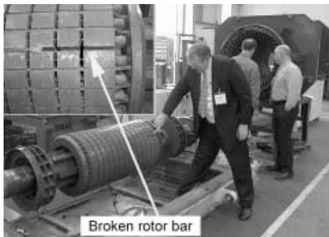
Figure 7. Broken Rotor Bar Lifted out of the Slot.
