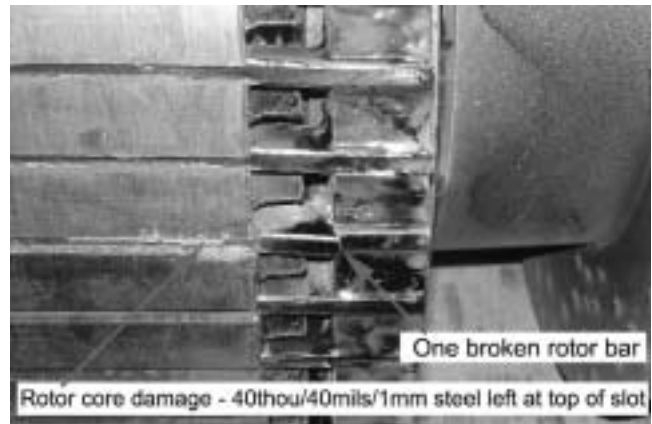
Figure 15. Faulty Rotor Winding Diagnosed via MCSA—Prevented Secondary Damage to HV Stator Winding.
