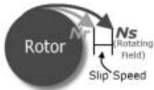
Figure A-1. Illustration of Slip Speed.
