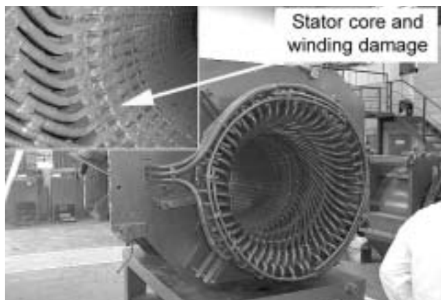
Figure 8. Mechanical Damage to HV Stator Winding.
