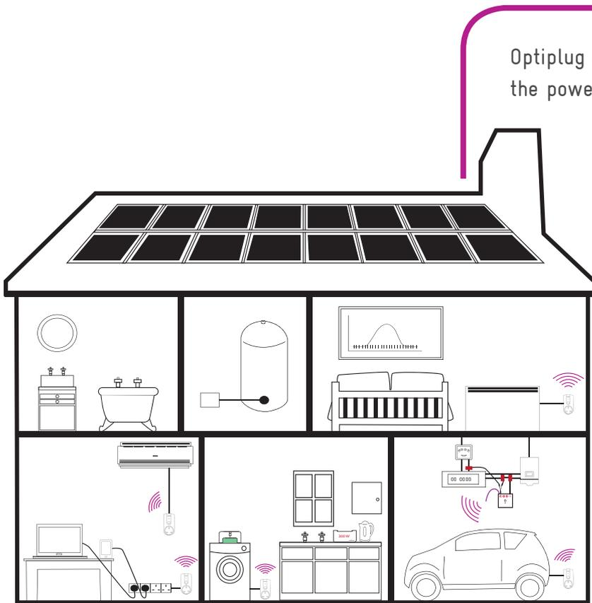
Optiplug uses Wattson sensors to constantly measure the power being generated by Solar PV and in use in the home. This information is transmitted over RF to the clever Optiplug system.
