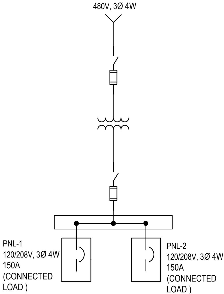
4. Based on the connected load of 150A, 120/208V 3 phase, 4W at each panel size the following:
