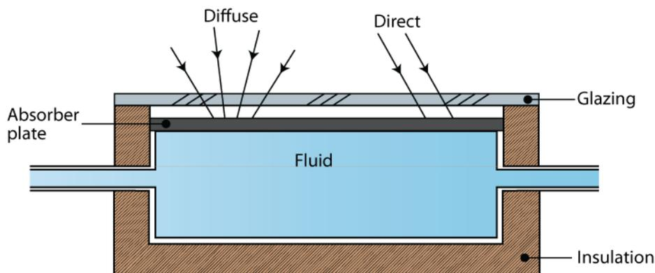
This is the most common panel for solar water heating
