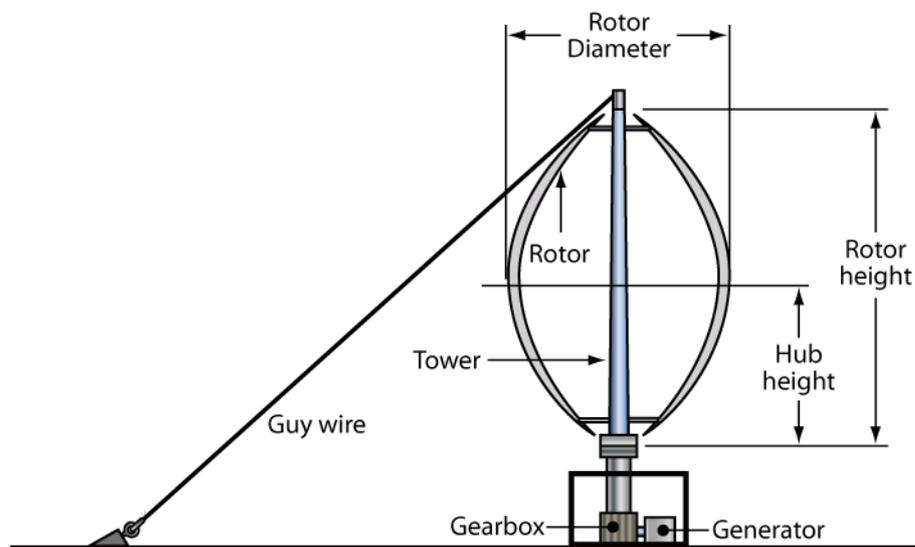
The other variant of the Darrieus type wind turbine looks more like an egg-beater, with the blades connected at the top and bottom of the shaft. Such a wind turbine is not generally self-starting and will usually require either mechanical brakes or other means of speed control as at a certain velocity resonance builds up leading to stress fractures.
