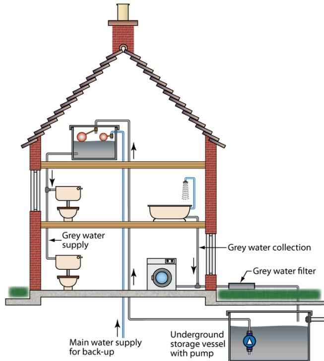
Grey water reuse systems vary significantly; however most have common features such as a tank for storing the treated water, a pump, a distributor system for transporting the treated water to where it is needed.
