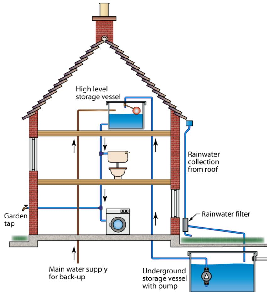
As water enters the tank it passes through a calmed inlet which calms the flow of water and prevents disturbance of the float switch and any sediments. Water is then supplied on demand by the submersible pump through a floating suction filter to specific outlets, usually WCs, washing machine and the like.
