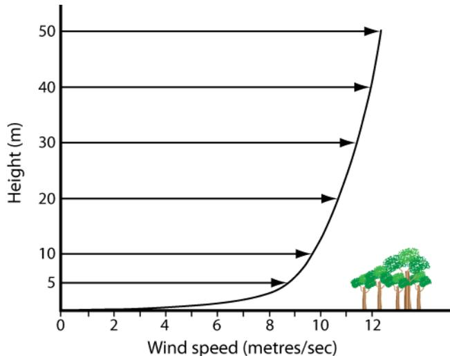
To this end the positioning of wind turbines is critical. Where the turbine is too near to the ground, the wind speed is reduced due to ground drag. Where turbines are in close proximity they may interfere with one another's air flow.
