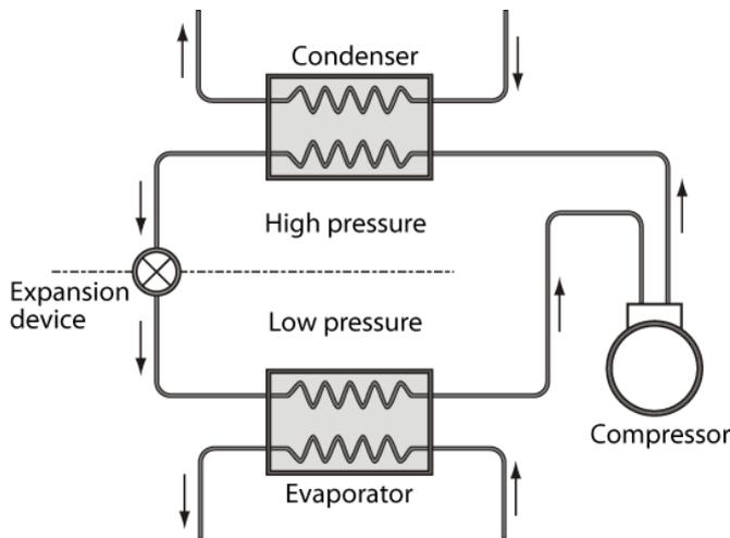
The majority of refrigeration systems are based on a machine which compresses and pumps refrigerant, such as R134a<sup>i</sup>, around a sealed circuit where heat is absorbed at low pressure and temperature and rejected at high pressure and temperature in heat exchangers.
