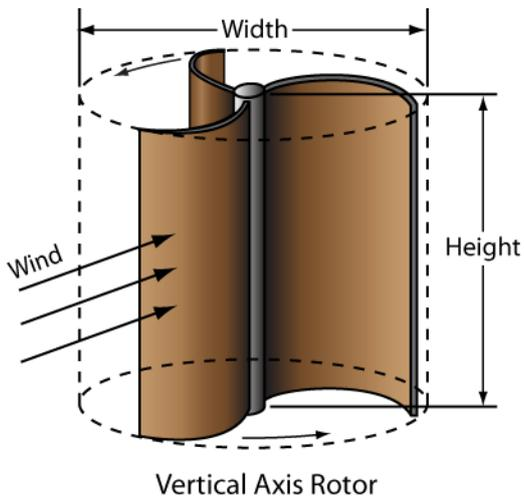
The Savonius wind turbine is the simplest type of wind turbine. They operate as a drag-type device like an anemometer. They are not efficient and are not always self-starting.
