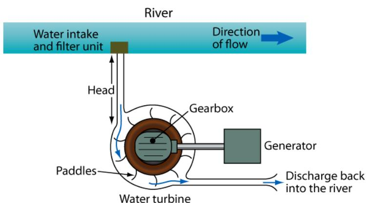
In this type of hydroelectric station, the water passes through the turbines that turn at 3000 rpm (revolutions per minute or 50 times a second). The water then passes out into a local river.
