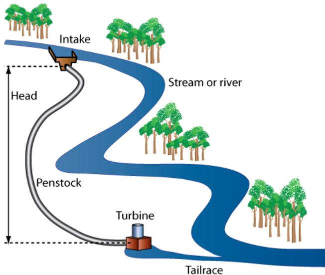
Hydropower systems that generate up to 100 kilowatts (kW) of electricity are often called micro-hydro systems.
