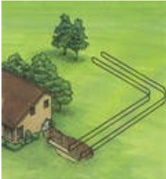
Ground source heat pumps take heat from the ground and release it in another location at a higher temperature.
