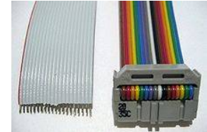
Insulation displacement
