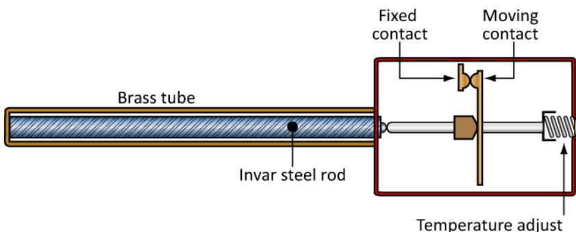
This type of arrangement is slightly different to the normal bi-metallic strip, but the principle of expanding materials at temperature is the same.
