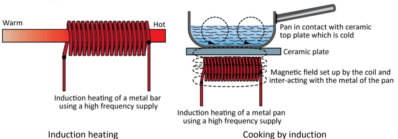
An induction heater for any process consists of an electromagnet, through which a high-frequency alternating current (a.c.) is passed.
