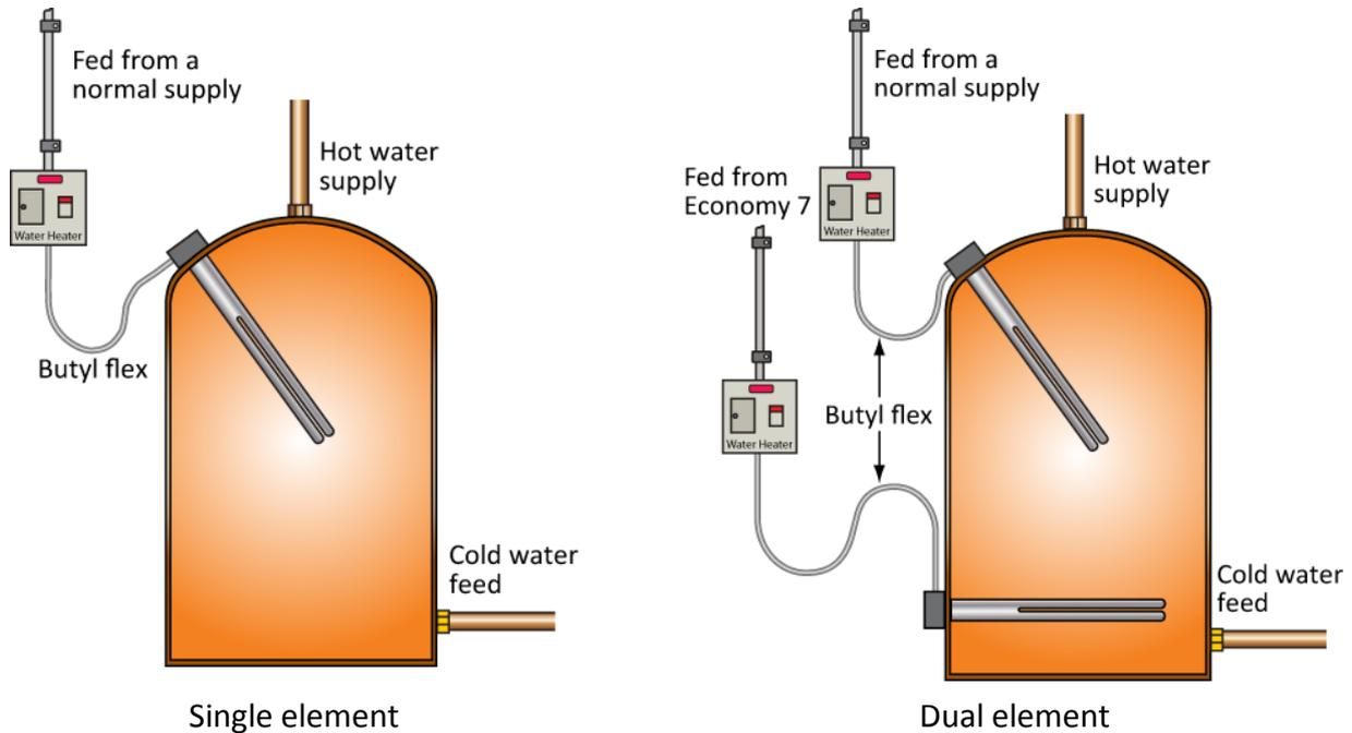
With the dual heater, a small element is used for heating just the top of the tank, and a large one for when more hot water is needed such as when running a bath, is placed at the bottom. This provides some flexibility. In reality the ideal position for the element is the bottom of the tank. With this arrangement it is more common that the larger element is controlled via an economy 7 tariff, whilst the smaller element is used for a daytime boost.
