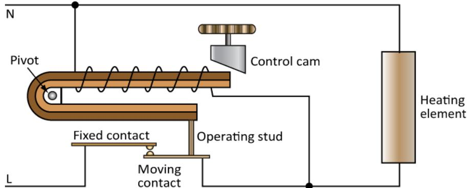
Here the simmer stat is a bimetallic strip wound with a coil. The coil around the bimetallic strip operates in tandem with the current passing through the cooker element.
