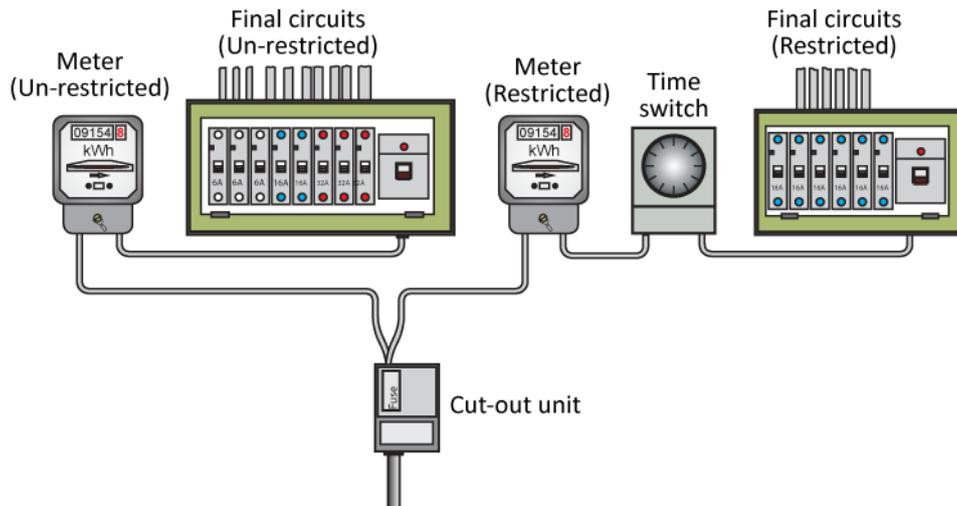
The other method still uses a time switch but uses one meter which has dual means of recording energy usage. This is more popular as the time switch is normally radio controlled by the distributor. This is done so that the distributor can vary the 7 hours of cheaper energy.
