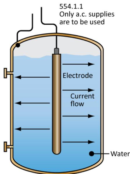
Water is covering the electrode which means that there is current flow
