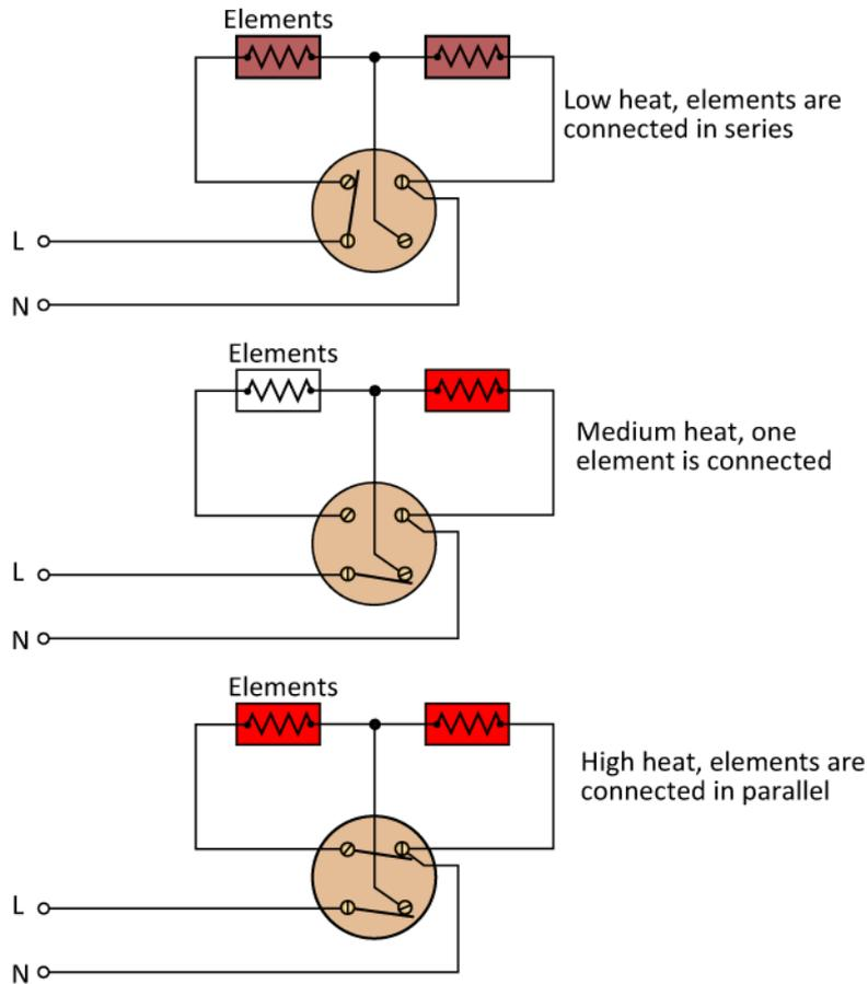
The first of the three diagrams shown above shows the cooker with both of the elements connected in series. This is the lowest setting
