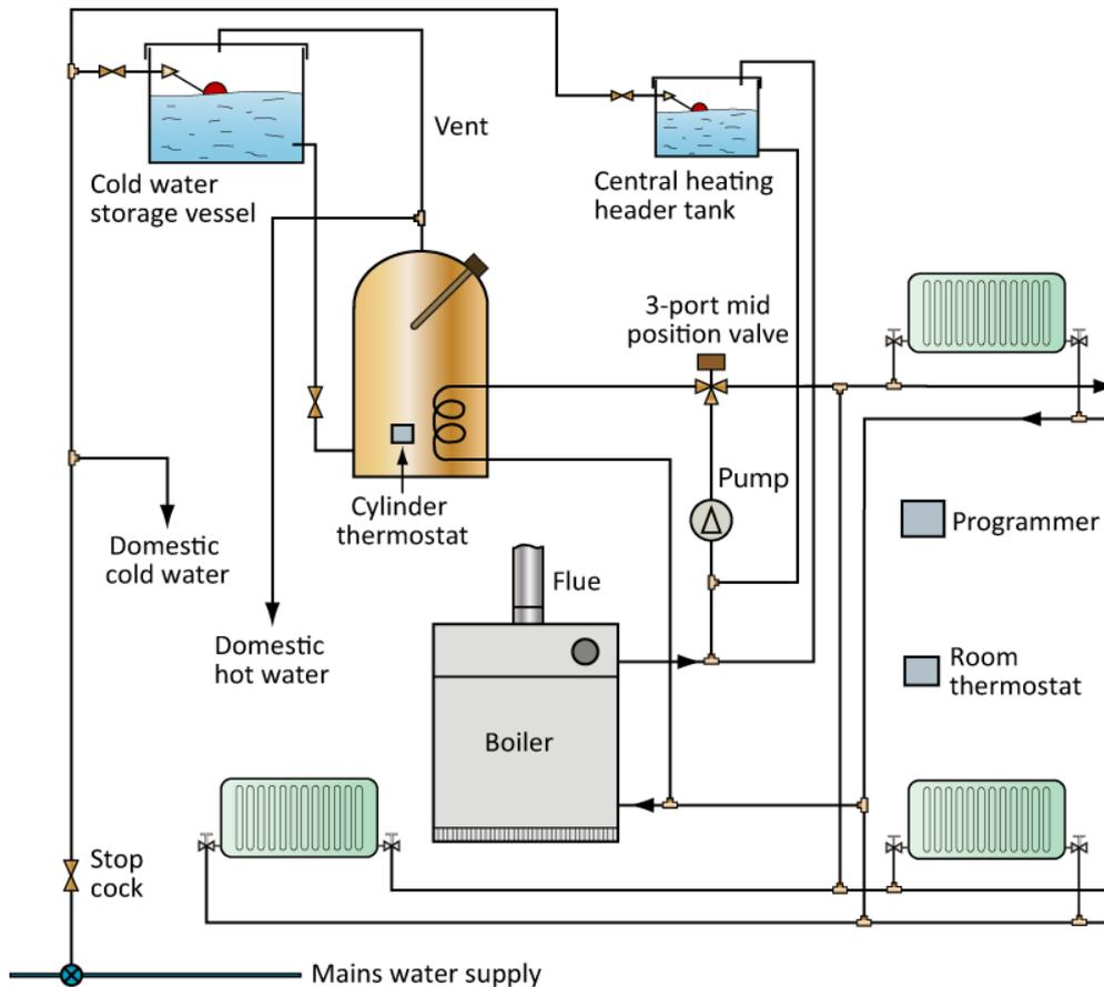
This is a fairly common type of arrangement and does satisfy the requirements of Part L of the Building Regulations if used with thermostatic radiator valves (TRV's). The disadvantages of this plan are that it doesn't allow for zoning of say the upstairs and downstairs rooms in larger houses, for this the S-Plan Plus must be used, and the flow rate through the mid-position valve is not as good as through a two port valve.
