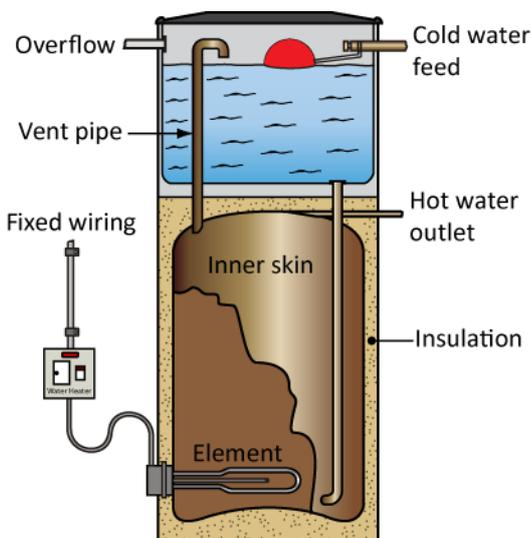
The immersion heater is usually placed in a large tank. This type of arrangement is a little smaller, although it is still capable of feeding a number of hand basins.
