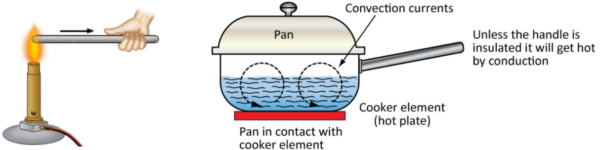
The end of the bar will get warm by the process of heat being conducted along its length.
