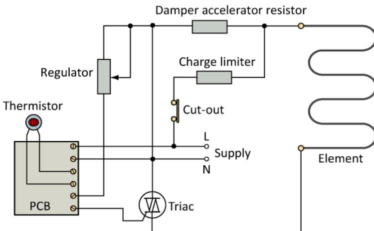
The cutout is a short-term means of limiting the problems of overheating and will either automatically reset or be reset by the press of a button.
