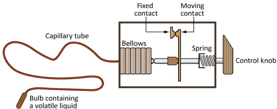
Here the tube is filled with a liquid that responds very readily to heat change. As the liquid expands then the bellows expand and break the contacts.
