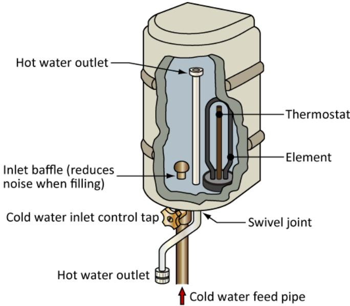
The water is heated via the element and controlled via the thermostat. The hot water, when required, will only flow when the cold-water tap is open. This quietly fills the heater because of the inlet baffle and pushes the heated water into the hot water outlet pipe.
