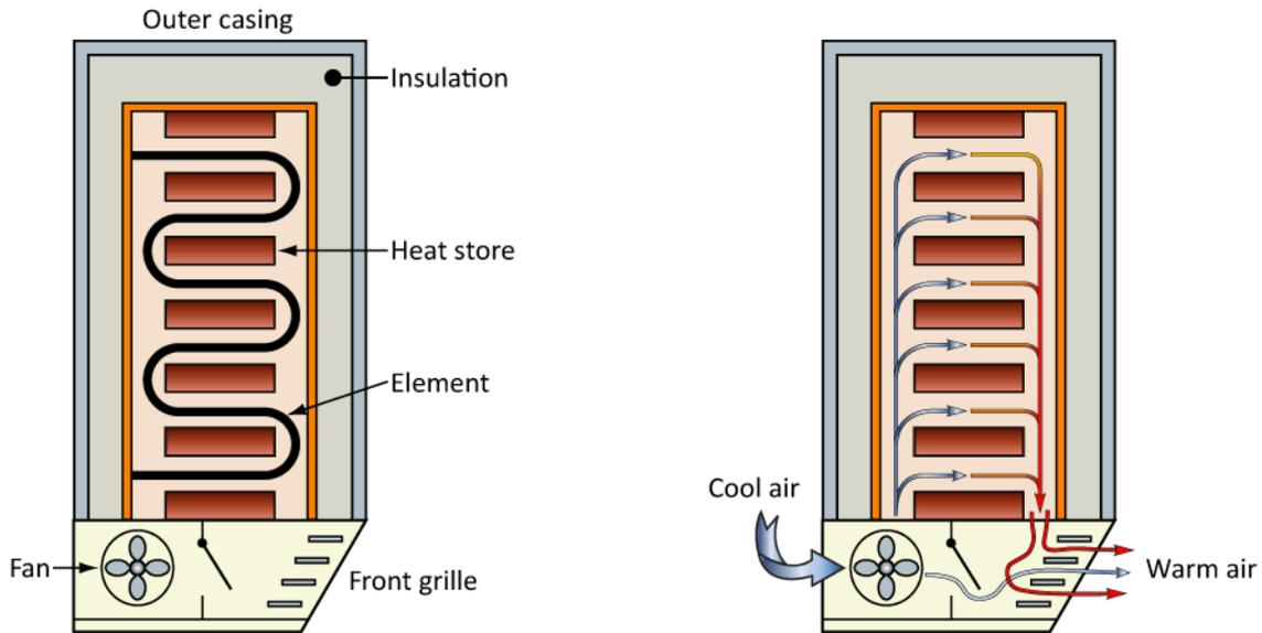
An Electricaire system consists of a central unit which can be a standalone unit or have a series of ducts attached to it which feeds each of the rooms with heated air. The units have a user control panel situated on the front so that the temperature can be manually controlled. These systems are usually complete and are supplied from off-peak electricity, such as economy7.
